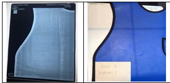
Picture 1 : test result lead apron quadrant 1 Apron A
